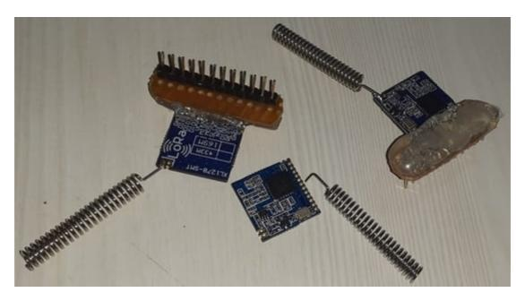
Now let us learn **SX1278 Arduino Interfacing**. For this, we will use two LoRa modules and two **Arduino Boards** to **send data** from one board and receive it on the other. We will use Arduino Nano at the **transmitter** side and Arduino Uno at the **receiver** side.
