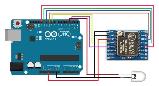
The LoRa SX1278 is not 5V friendly so do not supply 5V to it else the board will get damaged. Use 3.3V of Arduino to connect it to VCC pin. Connect all the GND pins to GND. Connect the RST pin to D9 and DIOo to D2 of Arduino. Connect the SPI Pins NSS, MOSI, MISO, SCK to Arduino D10, D11, D12, D13 of Arduino respectively as shown in circuit diagram above.
