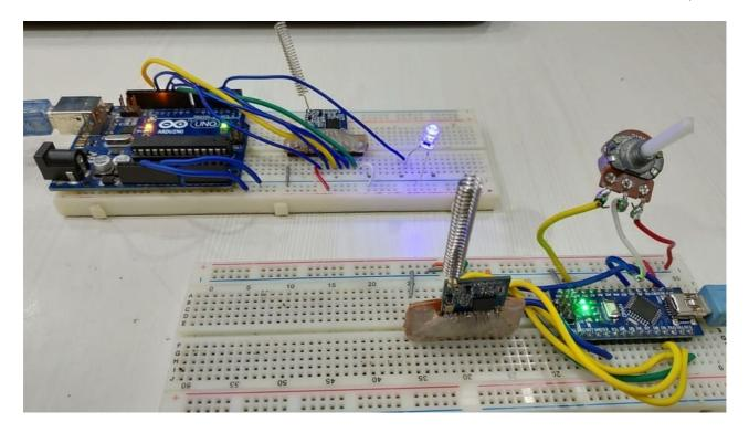
In this tutorial, we will learn about **Interfacing SX1278 (Ra-o2) LORA Module with Arduino**. We will see **SX1278 LORA & Arduino example** and make a **transmitter** & **receiver** circuit. We will control the brightness of LED wirelessly using potentiometer.
