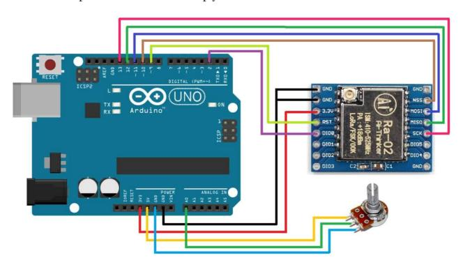
The LoRa SX1278 is not 5V friendly so do not supply 5V to it else the board will get damaged. Use 3.3V of Arduino to connect it to VCC pin. Connect all the GND pins to GND. Connect the RST pin to D9 and DIOo to D2 of Arduino. Connect the SPI Pins NSS, MOSI, MISO, SCK to Arduino D10, D11, D12, D13 of Arduino respectively as shown in circuit diagram above.
